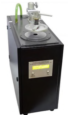
Fig. 2. Air permeability tester MT 160
