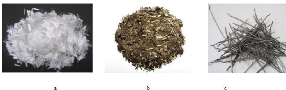
a – polypropylene fiber; b – basalt fiber; c – steel fiber
