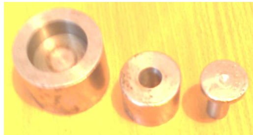
Fig. 3. The general view of the die, cylinder and piston of the mold
