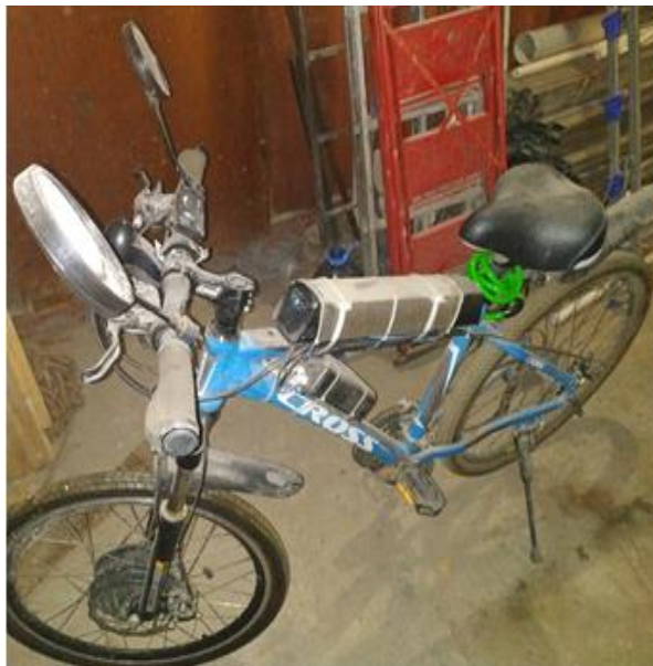
Figure 1. The appearance of two samples of an electric bicycle with an electric motor of 500 watts
